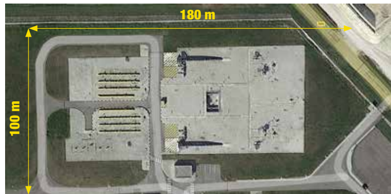
Aerial view of a valve, metering and regulation station comparable to the future BarMar receiving station.
